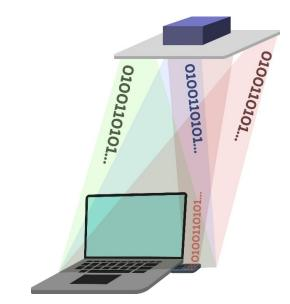
Fig. 2. Visible light communication system based on RGB LEDs.
